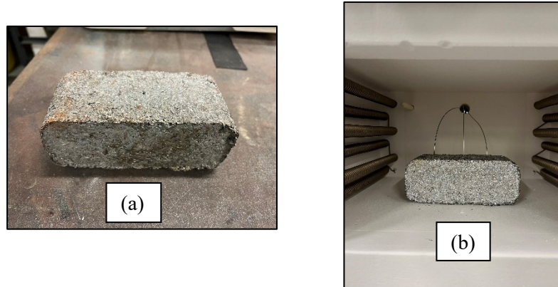
Figure 1 : (a) The aluminium scrap, (b) the aluminium scrap inside the oven
