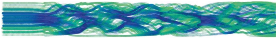
Fig. 1 hiVISC particle tracking results using PEPT. Particle positions are shown as an axial projection, coloured by velocity where high velocity is depicted darker than low velocity.
