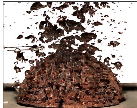
Figure 2. Topologically optimized 3D surface for pool boiling applications [2]
