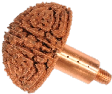
Figure 2. Topologically optimized 3D surface for pool boiling applications [2]
