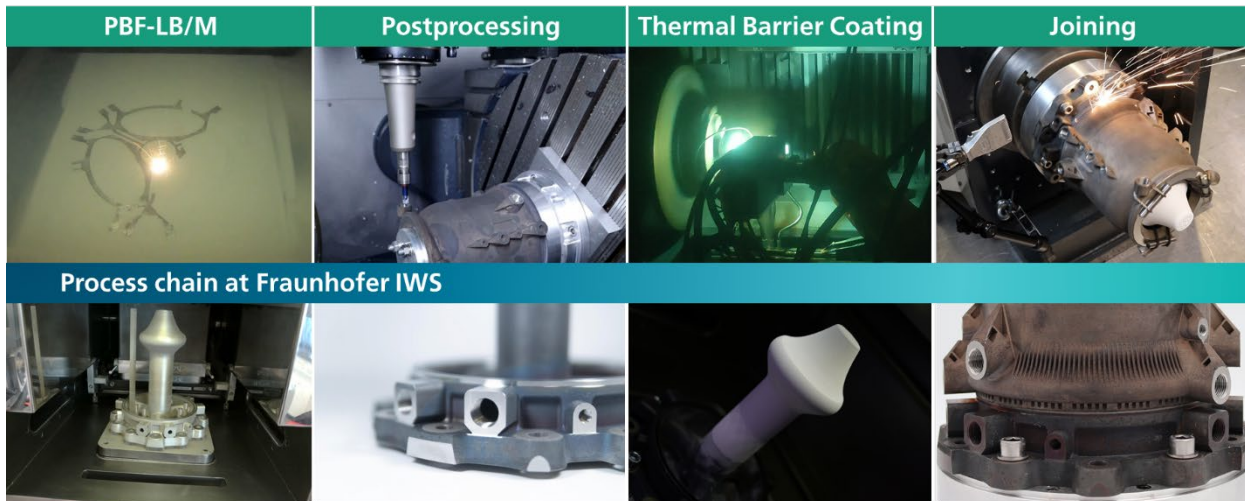
Fig. 1 Manufacturing route of the latest 6 kN aerospike breadboard engine (ASPIRER) at Fraunhofer IWS
