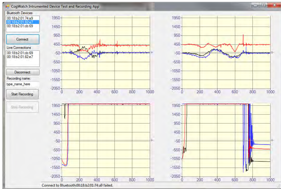
Figure 15 - Coaster test software with two connected coasters and their live data graphs.
