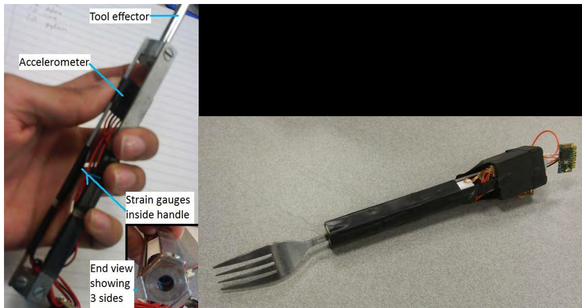
Figure 11 - Prototype handle dissection and prototype instrumented fork.
