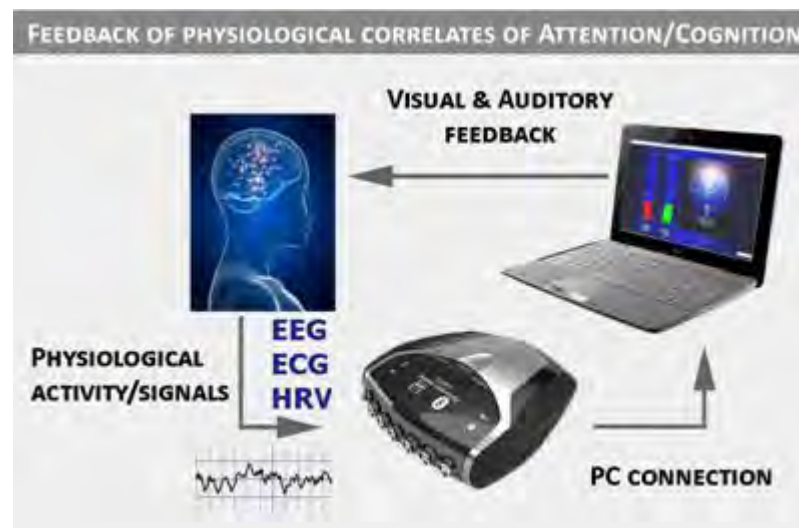
Figure 21: The CONTRAST setup for neurofeedback training.
