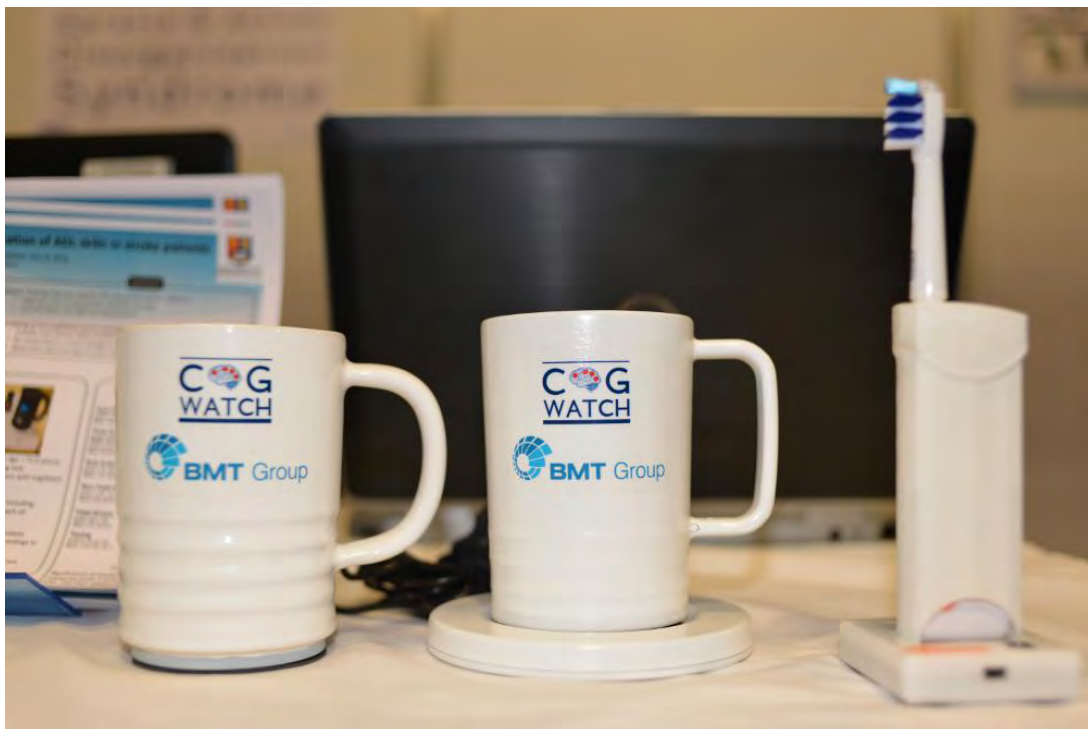
Figure 9: The final demonstrator of the one-size-fits-all concept coupled with a useable ceramic mug next to the sensorised toothbrush fitted with a shimmer sensor. From the exhibition at the UKSF2014 in Harrogate, UK.
