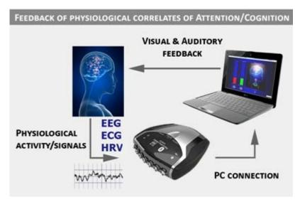
Figure 16. The CONTRAST setup for neurofeedback training.
