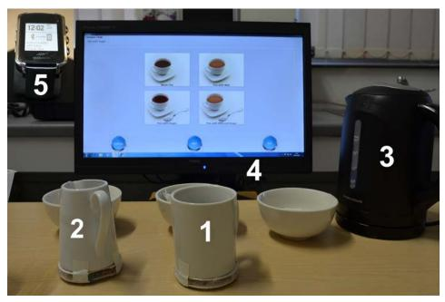
Figure 4. Prototype I (Patient side) components: 1) tea mug fitted with a sensorised coaster; 2) milk jug fitted with a sensorised coaster; 3) kettle fitted with gyroscope; 4) the VTE interface; the MetaWatch
