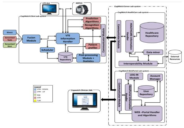
Figure 3. Global architecture of Prototype I including the *client* and clinician sides.
