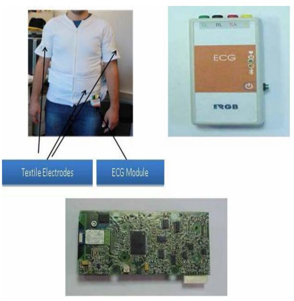
Figure 6. RGB hardware: module and electrodes.
