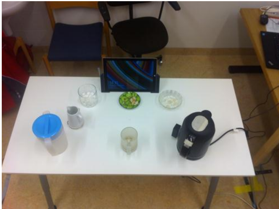
Figure 2. Test setup for tea-making. From left to right the objects included: a 300ml jug of water, jug of milk, sugar container, tablet computer (only used with the CogWatch System), plate for used tea-bags, cup, glass bowl containing new tea-bags and a kettle.
